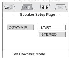
This is to activate the audio output from DOLBYAC3 5.1 DOWNMIX to 2 channel mode. Select the preferred SPEAKER connection by using the cursor buttons. Select the LT/RT to activate the Dolby surround compatible output. Select the STEREO to activate simple stereo mode.
